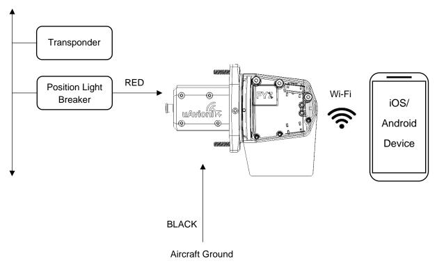
WARNING: Do not connect the power wire to a Xenon strobe power pack. This can damage the light and voids the warranty.
