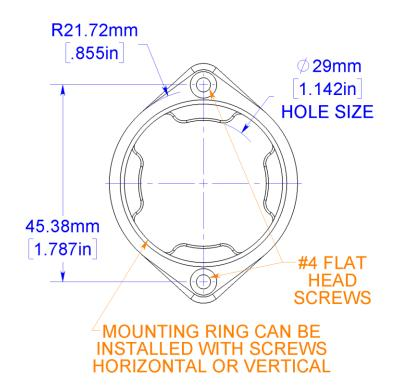
Determine if your aft position light is mounted vertical or horizontal.
