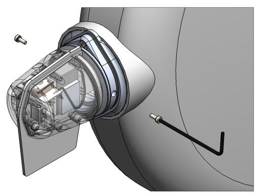
NOTE: THE UNIT SHOULD NOT REQUIRE MUCH FORCE TO ROTATE; IF YOU FEEL RESISTANCE WHEN ATTEMPTING TO ROTATE, STOP AND CONTACT SUPPORT. DO NOT INSTALL OR START THE ANTI-ROTATION SCREWS UNTIL AFTER THE UNIT IS INSTALLED AND ROTATED INTO POSITION.
