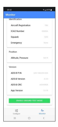
At this point, the technician can set the transponder mode back to "ALT" on the AV-30-C (Wi-Fi will be disabled) and the tailBeaconX will reply to Mode-S interrogations as if it was airborne. The tailBeaconX will also transmit airborne squitters accordingly.
