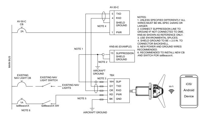
**6.3.2 Configuring the AV-30-C to Communicate with the tailBeaconX** After serial port wiring is complete, the AV-30-C must be configured to communicate with the tailBeaconX. This can be accomplished with the steps below.
