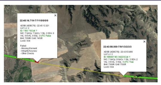
In the example above the aircraft callsign (ID), Mode A (M3), and emitter category (ECAT) are missing/invalid after the unit resumes transmission. The UTC sync is also *False*. The unit above is experiencing resets due to a power related event. The reset appears in the data as a loss of GPS reception but the supporting date indicates the skyBeacon/tailBeacon hardware momentarily lost power.
