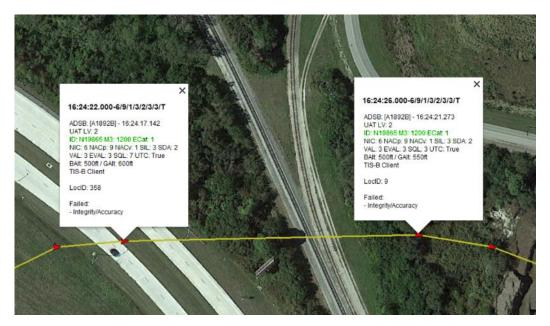
The data in both transmits above contains valid information on either side of the gap. No fields are missing or invalid which indicates the skyBeacon/tailBeacon hardware did not reset or lose power.
