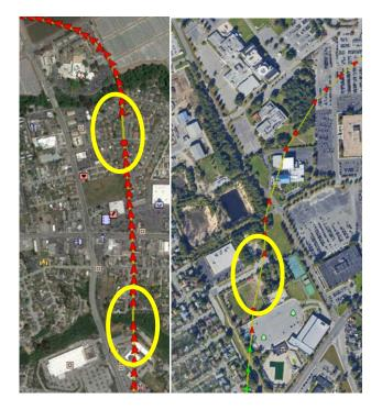
There are multiple causes of apparent GPS position loss. Further review is necessary to determine whether the loss of position is the result of a loss of GPS fix or a reset of the skyBeacon/tailBeacon hardware. A review of the ADS-B messages around the gap can be used to determine if the GPS lost position or the skyBeacon/tailBeacon reset due to a power event.
