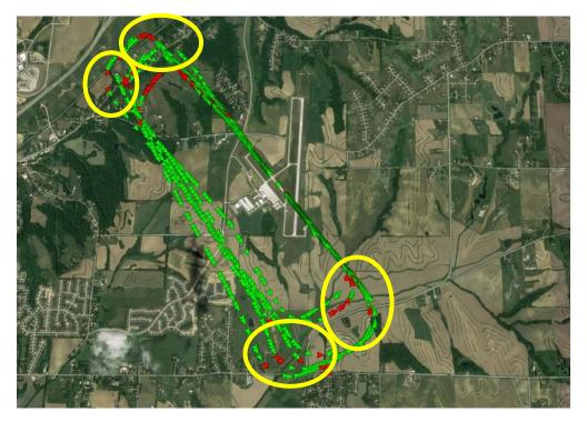
In the image above the GPS reporting fails integrity or loses position each time the COM radio is keyed. The positions of failure match normal call up locations during pattern work. This aircraft appears to be experiencing RF interference. See Section 5.2 for guidance on RF Interference troubleshooting.
