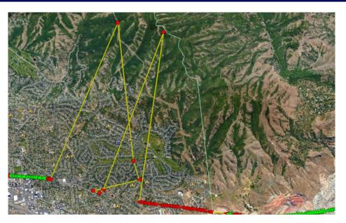
As shown above the flight track jumps unexpectedly and well outside the capability of the aircraft.
