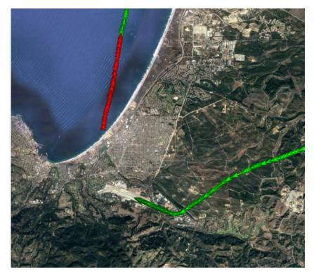
The aircraft above took off prior to having a high integrity fix. Turning on the navigation lights and skyBeacon/tailBeacon early in the aircraft runup helps prevent this type of failure.
