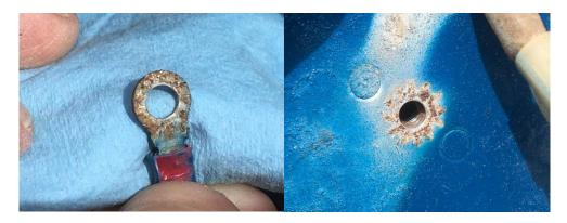
The photos of the above ring terminal and ground location show significant corrosion. The high resistance connection resulted in failure of the attached avionics. Removing the existing corrosion and existing paint/coatings along with replacement of the ring terminal resolved the performance issues.
