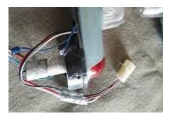
The photo above shows a series of wiring with three butt splices and a Molex plug on the same short section of power wiring. Presumably the mating side under the wingtip also has the same chain of wiring, compounding the chances of a failed connection and increasing the resistance. If both sides of the installation have three additional butt splices there are a total of twelve additional and unnecessary failure points.
