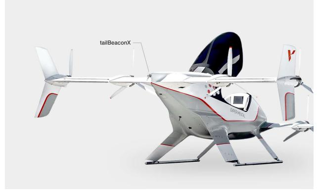
tailBeaconX is the first transponder to be specifically evaluated by Aireon and NAV CANADA, early tests are showing promise toward meeting performance requirements for ATC-quality surveillance data for GA aircraft. "A solution like tailBeaconX will expand the proven safety and operational benefits of ADS-B through a space-based service to the general aviation community," said Cyriel Kronenburg, Vice
