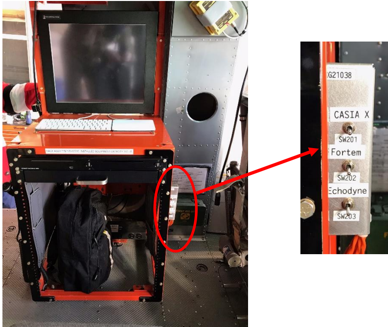
Figure 4: Engineering Workstation power switches
