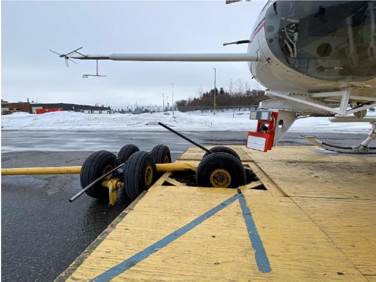
Figure 23: Radar clearance with platform tire
