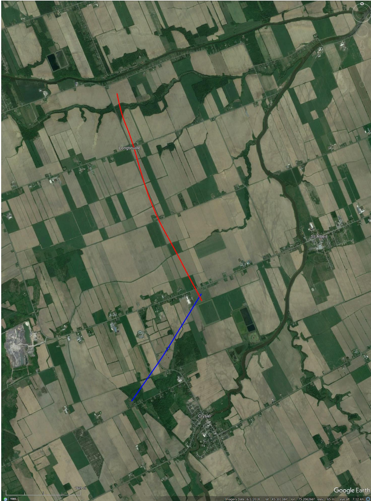
Figure 24: Example Flight Path from Intercept 15 -32 Degrees Azimuth (Blue - Bell 205, Red - Harvard)
