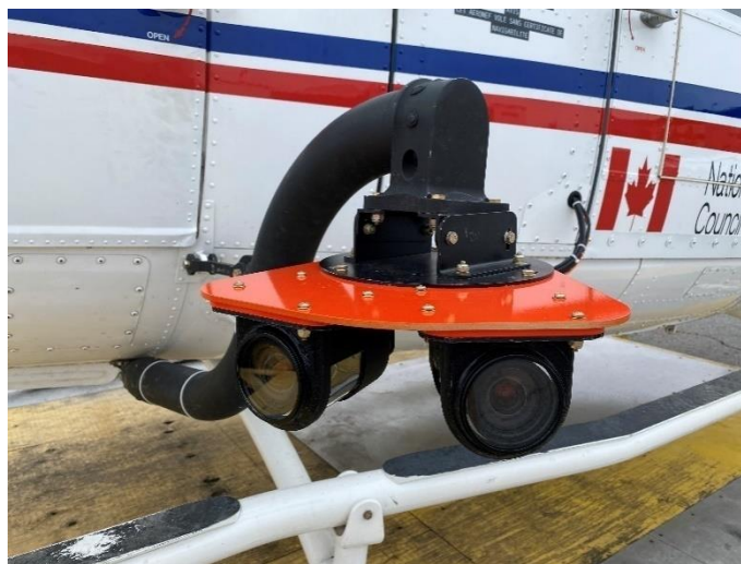
Figure 18: Casia X Camera Installation
