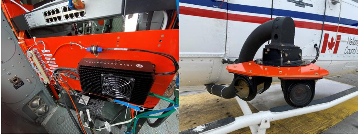
Figure 2: CASIA Camera Module (L) and CASIA Cameras on FLIR Mounting Arm (R)
