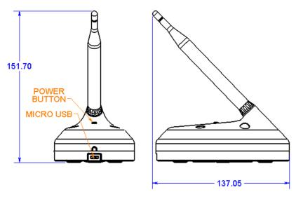
ny antenna certified to TSO-C66, TSO-C74, TSO-C112 with a peak gain of 4 dBi or less, a omni-directional radiation pattern, and a VSWR of 1.8 or less at 978MHz is approved for use 20gr25with this device and will ensure conformance to all applicable standards for RF emissions. Ensure that the polarization of the antenna is as near vertical as possible.
