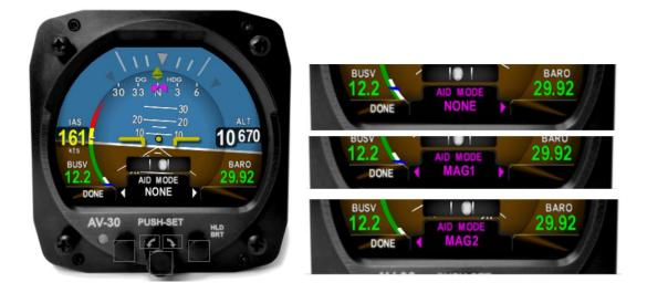
The factory setting for non-magnetometer equipped units is NONE, and the factory setting for magnetometer equipped units is MAG1. Leave the AID Mode set to the default, unless otherwise direct by uAvionix Support.
