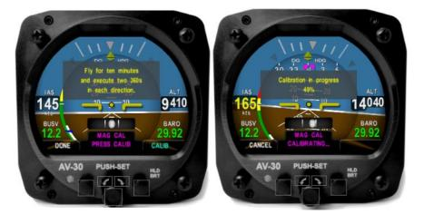
3. Fly for 10 minutes. Four, 360-degree standard rate turns will need to be completed. Each turn will represent 25% of the total.
