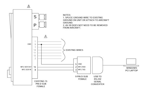
Note: AV-Link must not be installed if performing an update using the PC serial update procedure.
