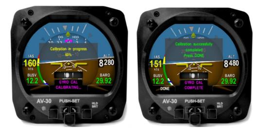
AV-30-E will indicate "Calibration successfully completed Press DONE".
