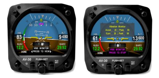
Record the data on the screen to share with uAvionix Support. Push the center button again to stop monitoring vibration and return to the Installation Menu.
