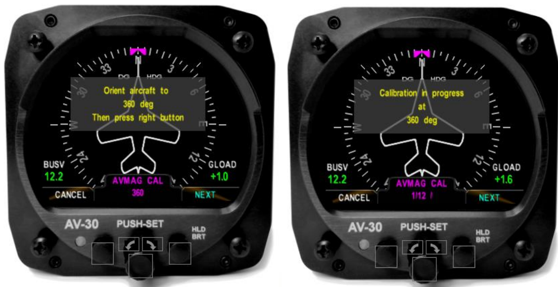
Figure 52 – AVMAG CAL In-Progress
