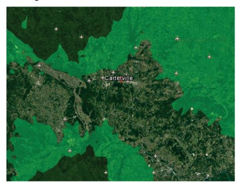
At 500AGL the radar (dark green) and ADS-B (light green) coverage are both non-existent. Depending on the field the aircraft departed from, and the direction of flight, a large gap and random failures are very likely. The data from the PAPR and the coverage map all support the fact that this flight likely failed due to coverage issues and not configuration or defective equipment. Detailed data can be requested to verify
